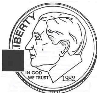
Figure 4-1. A chip compared to a dime. This incredibly tiny microchip, the brain of an entire computer, is equivalent to 450,000 transistors.
